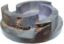
Figure 11 - The damaging effects of cavitation
