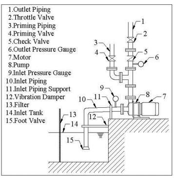
Figure 6 - Effective piping design will minimize life cycle costs
