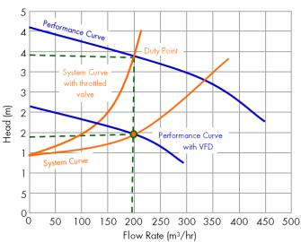
Figure 7—Achieving a desired duty through a throttle valve instead of a VFD
