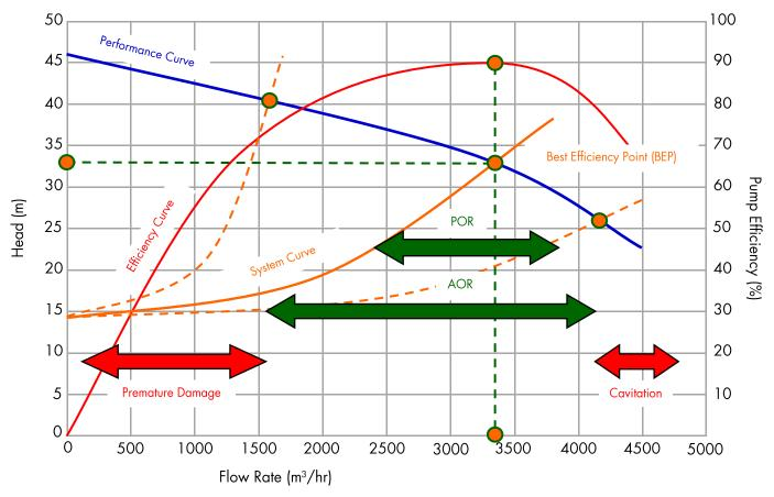
Figure 4 - Operating at the BEP maximises efficiency and operational life
