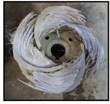
fluid in the Figure 9 - Running a pump dry can quickly result in a costly repair bill
